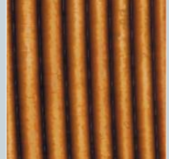
Images of MO disk Topographic image (left) Magnetic force image (right)
