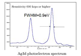
Monochromatic X-rays are ideal for high resolution analysis. The figure on the left
