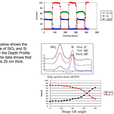
The figure below shows the depth profile of SiO<sub>2</sub> and Si obtained by the Depth Profile program. The data shows that each layer is 25 nm thick.
