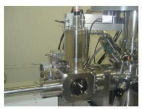
The high speed ion gun is specifically designed for XPS to etch samples at a low accelerating voltage from 150 V to 1500 V, minimizing the damage on the surface and interface. The etching rate is 3 to 120 nm/min (SiO<sub>2</sub> conversion).
