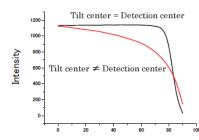
When the detection center differs from the tilt center, the sample height will change in one direction relative to the tilt, and so will the peak intensity. When the detection center coincides with the tilt center, the sample height will change in both directions. offsetting the changes in peak intensity.
