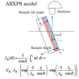
CA: Concentration distributions in t1 and t2 layers  $\lambda$  A: Mean free path of electrons emitted from 2<sup>nd</sup> layer
