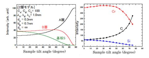
The resulting profile and the curve from model calculation were compared to estimate the thickness of the layer structure. The figure on the left shows the calculated intensity of each layer, while the figure on the right shows the measured results.
