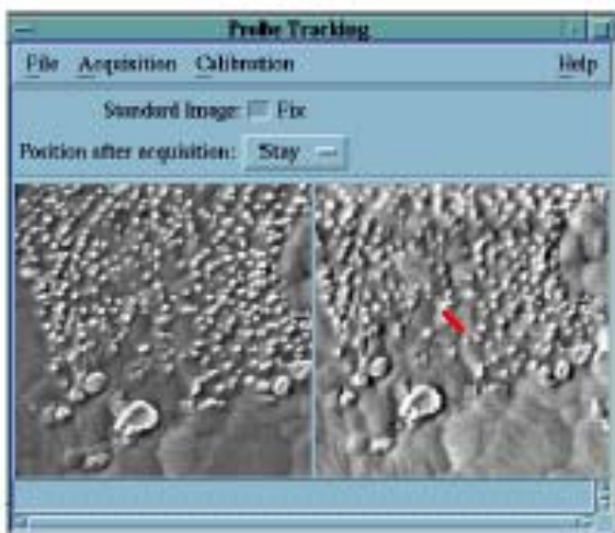
Secondary electron image (512 × 512 pixels) Sample: Lead free solder
